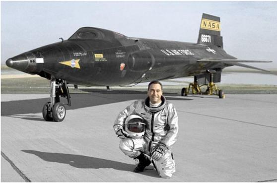
*Air Force test pilot William J. "Pete" Knight with X-15 aircraft number 56-6671. This photo was before Knight's speed record flight when the X-15 received a white, heat-resistant coating. Photo Credit: NASA.*
