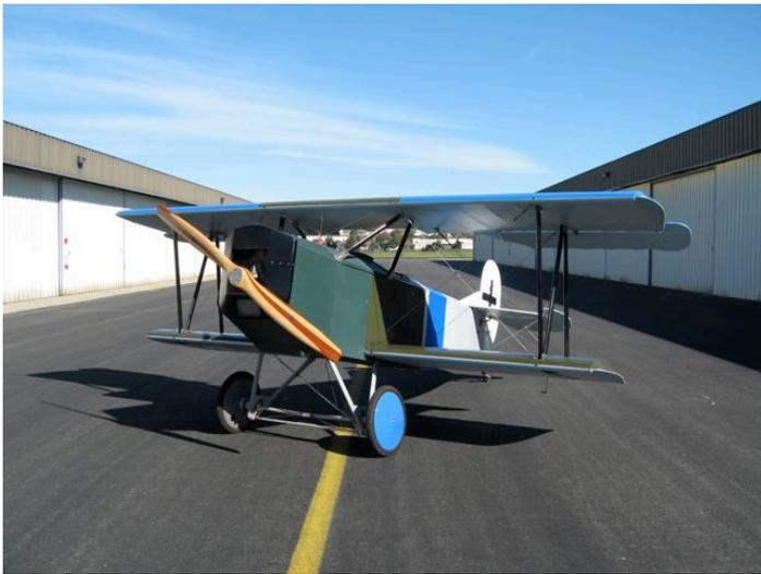
General handling is very similar to Travis Gier's Dr. 1 When I remove my feet from the rudder pedals at cruise, the aircraft tracks straight, with no yaw instability. Removing my hand from the stick, the aircraft flies straight and level (if the fuel load AND mine are just right!) Control forces are light, but not "twitchy." Stalls result in a "mush" (no real break) but a HUGE sink rate. This aircraft seems to have the glide ratio of a DROPPED rock-- VERY LOW INERTIA!!
